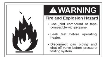
Use pipe joint compound or teflon tape marked as being resistant to the action of petroleum (Propane [L.P.]) gases.
